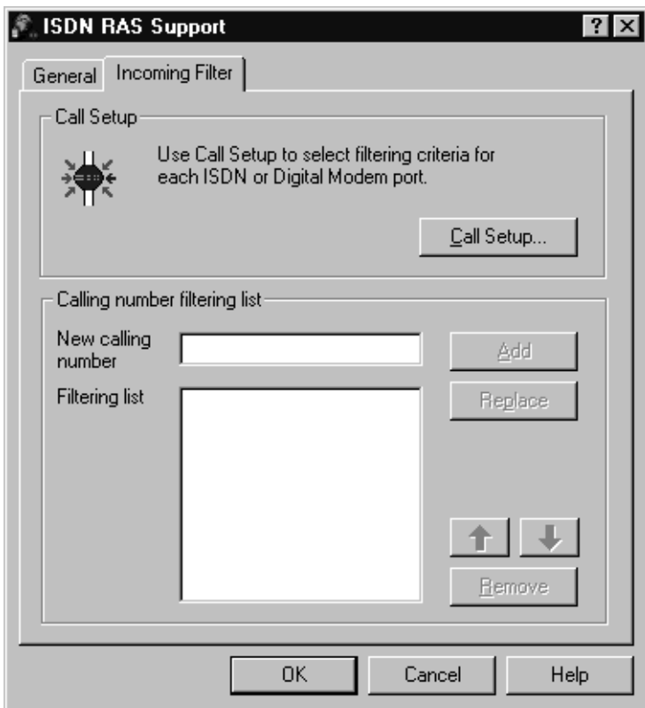
Figure 6-5. RAS Support Incoming Filter Dialog Box
