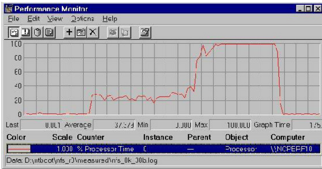
Figure 5. CPU Utilization: 30 Network Stations using NFS, 8 KB blocks, & Single 10-Mbit LAN. Time scale used is 7 seconds per horizontal unit.
