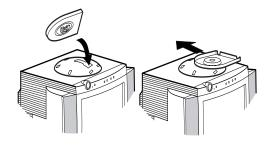
3 Turn the interface 90° counter clockwise as shown in the next diagram.
