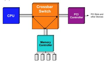
Figure 8. Crossbar switch architecture.
