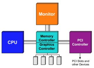
Figure 6. Unified Memory Architecture used in the 02 workstation from Silicon Graphics, Inc.
