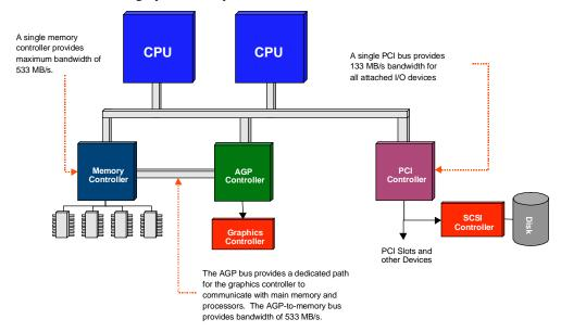
Figure 9. Block diagram of the LX architecture.
