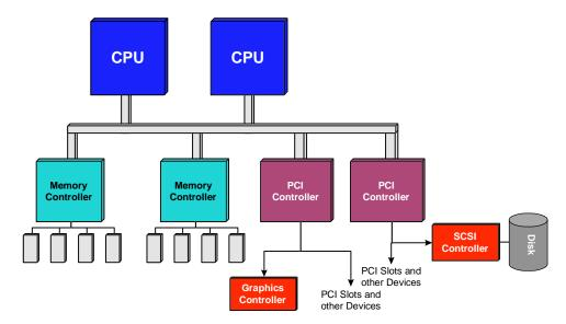
Figure 7. The new Highly Parallel System Architecture allows the processors and graphics controller to access two separate memory buses concurrently.
