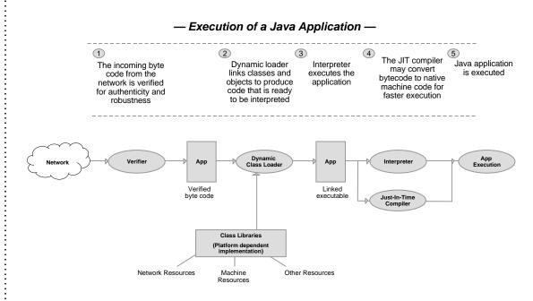
The Java runtime environment consists of a bytecode verifier, a class loader, a virtual machine, and an optional Just in Time (JIT) compiler.
