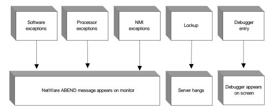
Figure 3. Server failure with the NetWare ABEND feature
