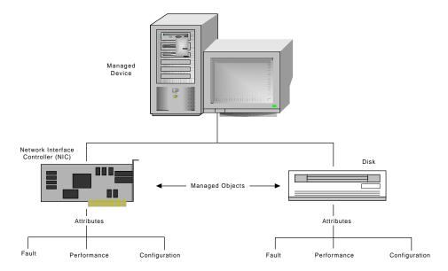
Figure 2. Managed device and its manageable objects
