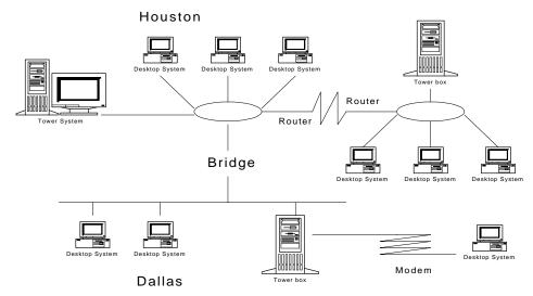
Figure 1. A typical computing network that includes both infrastructure and computing devices
