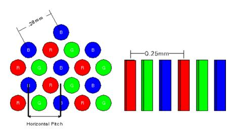
In aperture grille CRTs, the pitch is measured either on the phosphor (stripe pitch) or is measured on the wire, when it is defined as the grille pitch.
