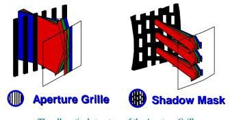
The all-vertical structure of the Aperture Grille permits more beams to reach the phosphor screen
