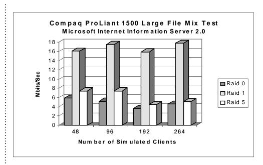
The chart above illustrates the disk subsystem impact on performance in the Compaq ProLiant 1500. Clearly RAID 1 outperforms the single drive spindle and the drive array configured with RAID 5 fault tolerance. RAID 1 outperforms RAID 5, providing a 30 to 50 percent increase in throughput. RAID 5 outperforms the single drive by approximately 20 percent.
