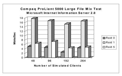
The chart above illustrates the disk subsystem impact on performance in the Compaq ProLiant 5000. Clearly RAID 1 outperforms the single drive spindle and the drive array configured with RAID 5 fault tolerance. RAID 1 outperforms RAID 5 providing from 2 - 3.5 times the throughput. RAID 5 outperforms the single drive to a less significant degree.
