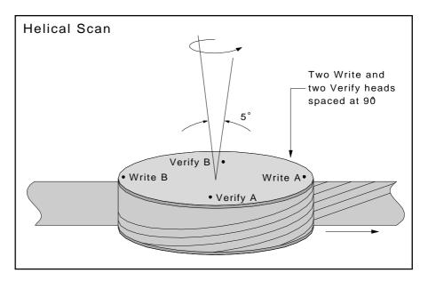
Figure 1. Helical-Scan Heads and Tape with Diagonal Tracks
