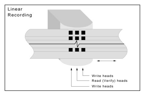
Figure 2. DLT Multiple Horizontal Tracks
