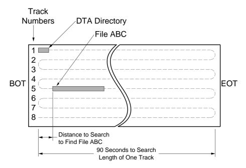
Figure 3. DLT Serpentine Track Layout
