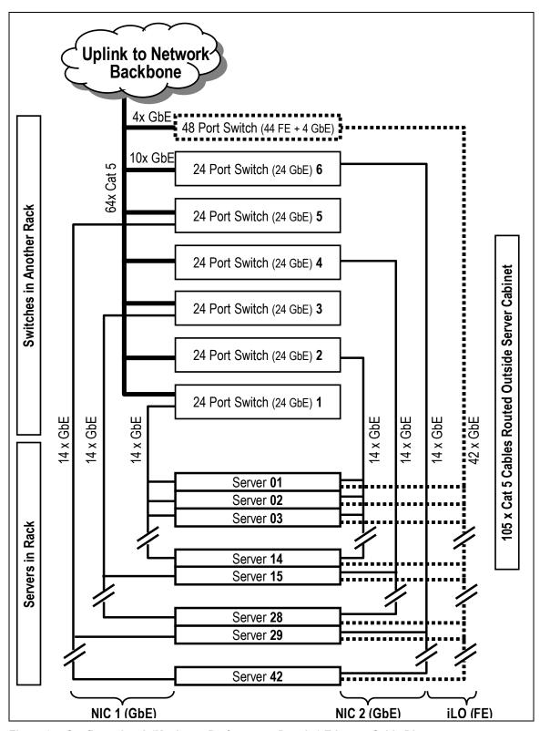
Figure 3. Configuration A (Maximum Performance Density) Ethernet Cable Diagram
