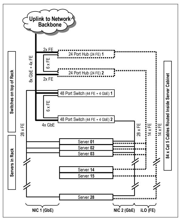
Figure 8. Configuration C (Traditionalist) Ethernet Cable Diagram
