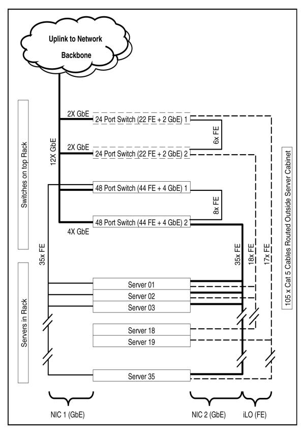
Figure 5. Configuration B (Maximum Flexibility) Ethernet Cable Diagram
