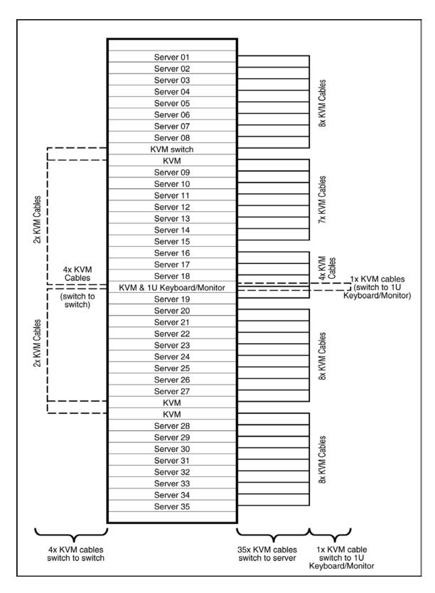
Figure 6. Configuration B (Maximum Flexibility) KVM Diagram
