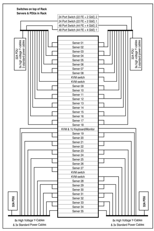
Figure 4. Configuration B (Maximum Flexibility) Power Diagram
