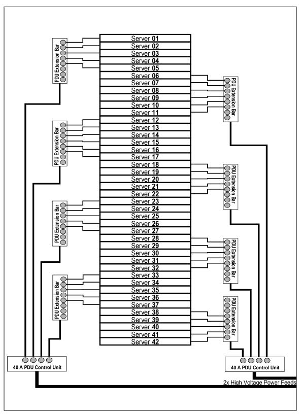
Figure 2. Configuration A (Maximum Performance Density) Power Diagram
