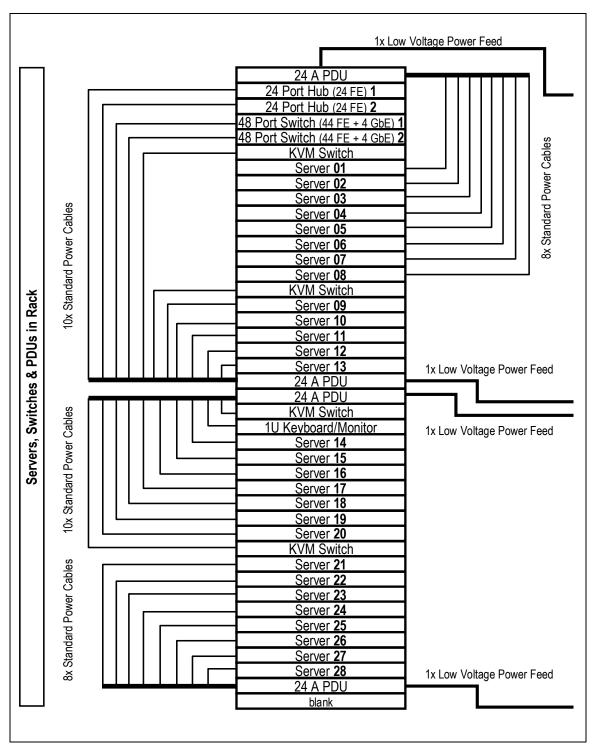
Figure 7. Configuration C (Traditionalist) Power Diagram
