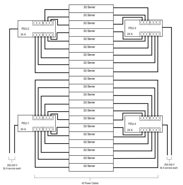
Figure 1. Four high-voltage PDUs (24A)
