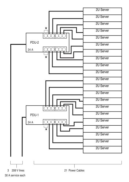
Figure 2. Two high-voltage PDUs (24A)
