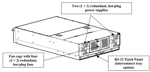
Figure 2. ProLiant BL e-Class server blade enclosure (rear view) with two redundant, hot-plug power supplies, fan cage with 4 redundant, hot-plug fans, and RJ-21 Patch Panel
