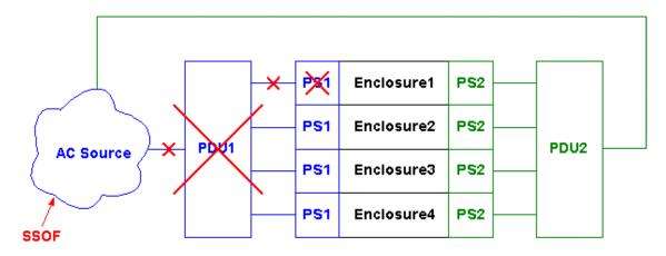
Figure 8. PDU redundancy, single source of failure = AC source
