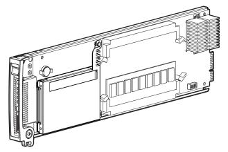
Figure 2. ProLiant BL10e single-processor server blade
