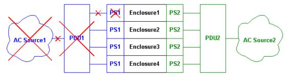
Figure 9. AC source full redundancy
