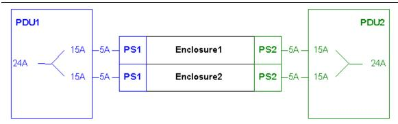
Figure 15. Low-line redundant PDU configuration supporting one to two enclosures
