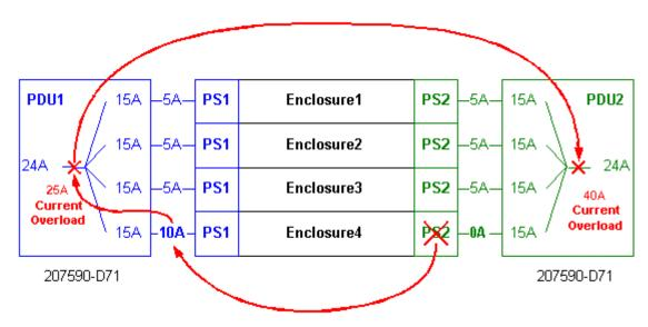
Figure 11. Domino effect caused by low-line current overload
