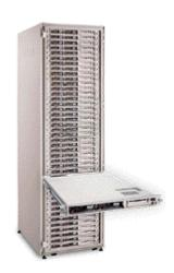
The ProLiant DL360 offers a solution for customers focused on saving space in the data center but planning to scale their environment by adding servers in the tens, hundreds, or even thousands. Its incredible, ultra-thin 1U chassis houses up to two 1.14GHz Pentium III processors in both single pack and 3-pack SKUs, 128 MB of 133-MHz ECC registered SDRAM DIMM memory expandable to 4 GB, and a 133-MHz GTL bus to deliver uncompromising performance.
