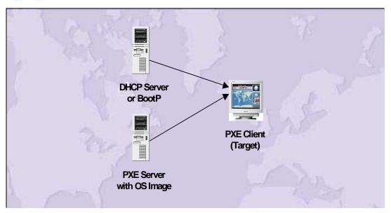
Figure 1. Typical PXE setup for Red Hat 6.2 Linux
