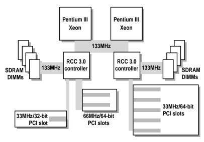
Figure 2. Highly parallel PCI bus architecture in the ProLiant ML530
