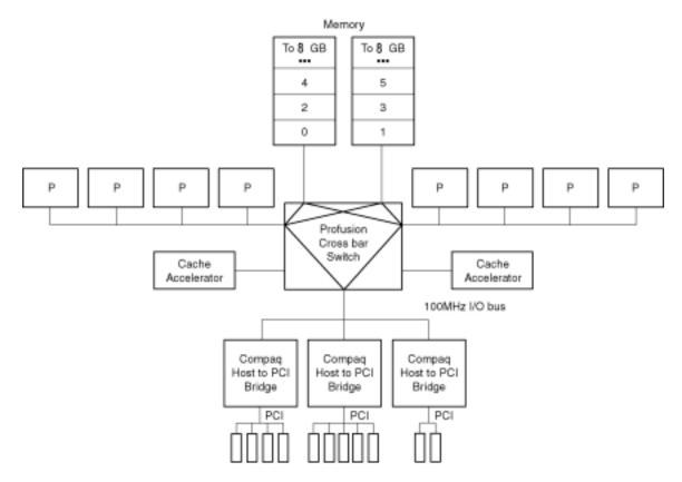
Figure 3. Triple-peer PCI bus architecture in the ProLiant 8000
