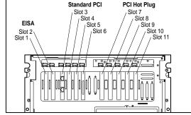
Figure 15. Location of expansion slots in rear of the ProLiant 6000 and 7000
