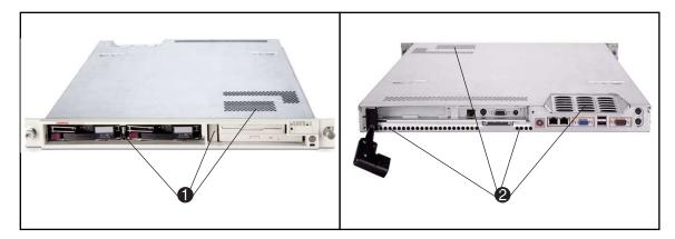
Figure 7: Intake 1 and Exhaust 2 vents for the ProLiant DL360 server
