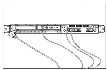
Figure 10: Typical cabling using the Remote Insight Lights-Out Edition (DL360 shown)
