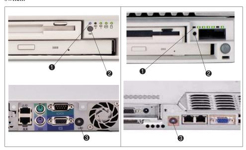
Figure 15: Unit Identification (UID) LEDs and switches (DL320 on left and DL360 on right)
