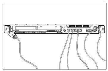
Figure 11: Typical cabling using server console switches (DL360 shown)
