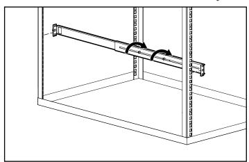
Figure 8: Compaq Third-Party Rack Option Kit rack rail depth adjustment
