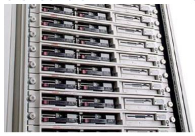
Figure 1: Deployment of 1U ProLiant DL360 ultra-dense servers in a cabinet rack
