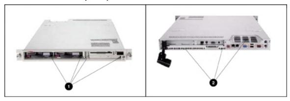
Figure 5: Intake and Exhaust vents for the Compaq ProLiant DL360 server
