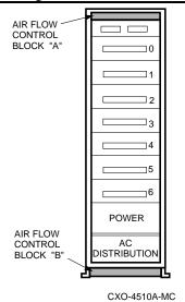
Baffle Install this baffle in the base of a single pedestal.
