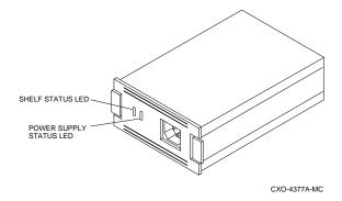
Figure 4-2 3.5-Inch SBB Status LEDs
