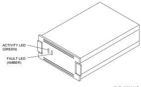
Figure 4-3 5.25-Inch SBB Status LEDs
