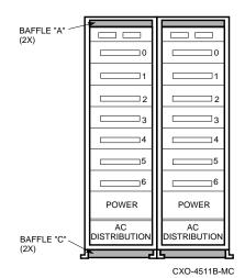
Baffle C Install this baffle in the base when using a multiple pedestal configuration.
