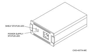
Figure 3-6 SBB Status LEDs
