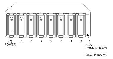
These shelves can accommodate either 3.5-inch or 5.25-inch StorageWorks building blocks (**SBB**s) in various combinations to create a storage array specifically suited to your needs. The SCSI bus controller capabilities can restrict the number of SBBs, the SBB types, and the combination SBB types you install.
