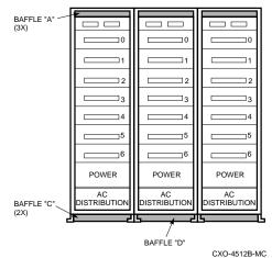
Baffle Install this baffle when using a multiple pedestal configuration (three or more pedestals).
