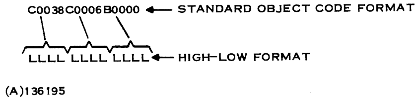
Figure 11-3. Standard Object Code Format to High-Low Format Conversion
