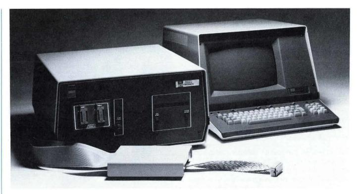
The 8001 Microprocessor Lab consists of the 8001 mainframe; an optional system terminal (TEKTRONIX CT8100 or CT8101 recommended); and a Microprocessor Support Package for the microprocessor selected. A support package includes an emulator ROM, an emulator processor, and a prototype control probe.
