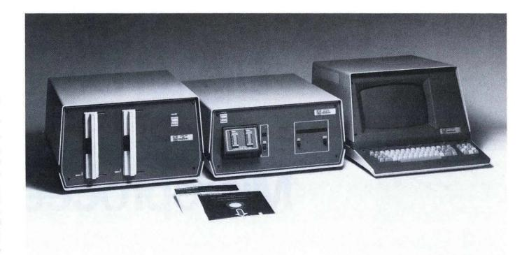
The 8002 Microprocessor Lab consists of the 8002 mainframe; the dual flexible disc unit; an optional system terminal (TEKTRONIX CT8100 or CT8101 recommended); and two sets of assembler software for two different microprocessors, chosen from the microprocessors supported at time of purchase. An emulator processor module for each microprocessor the system supports, and its associated prototype control probe, are offered as options.
