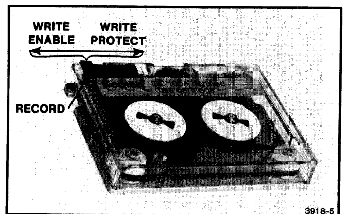
Figure 2-4. DC-100 Magnetic Tape Cartridge Write-Protection.
