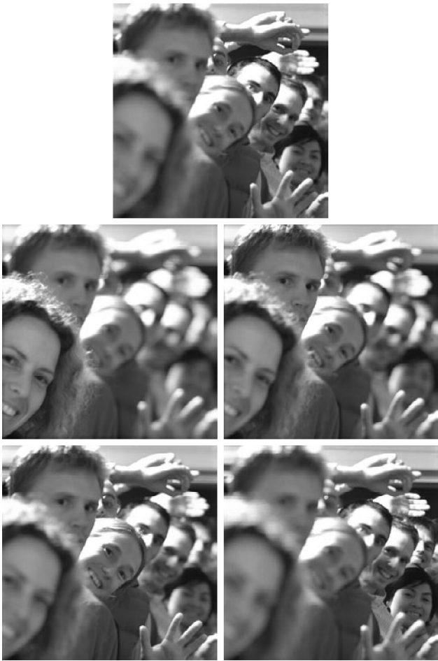
Figure 14: Refocusing after a single exposure of the light field camera. Top is the photo that would have resulted from a conventional camera, focused on the clasped fingers. The remaining images are photographs refocused at different depths: middle row is focused on first and second figures; last row is focused on third and last figures. Compare especially middle left and bottom right for full effective depth of field.
