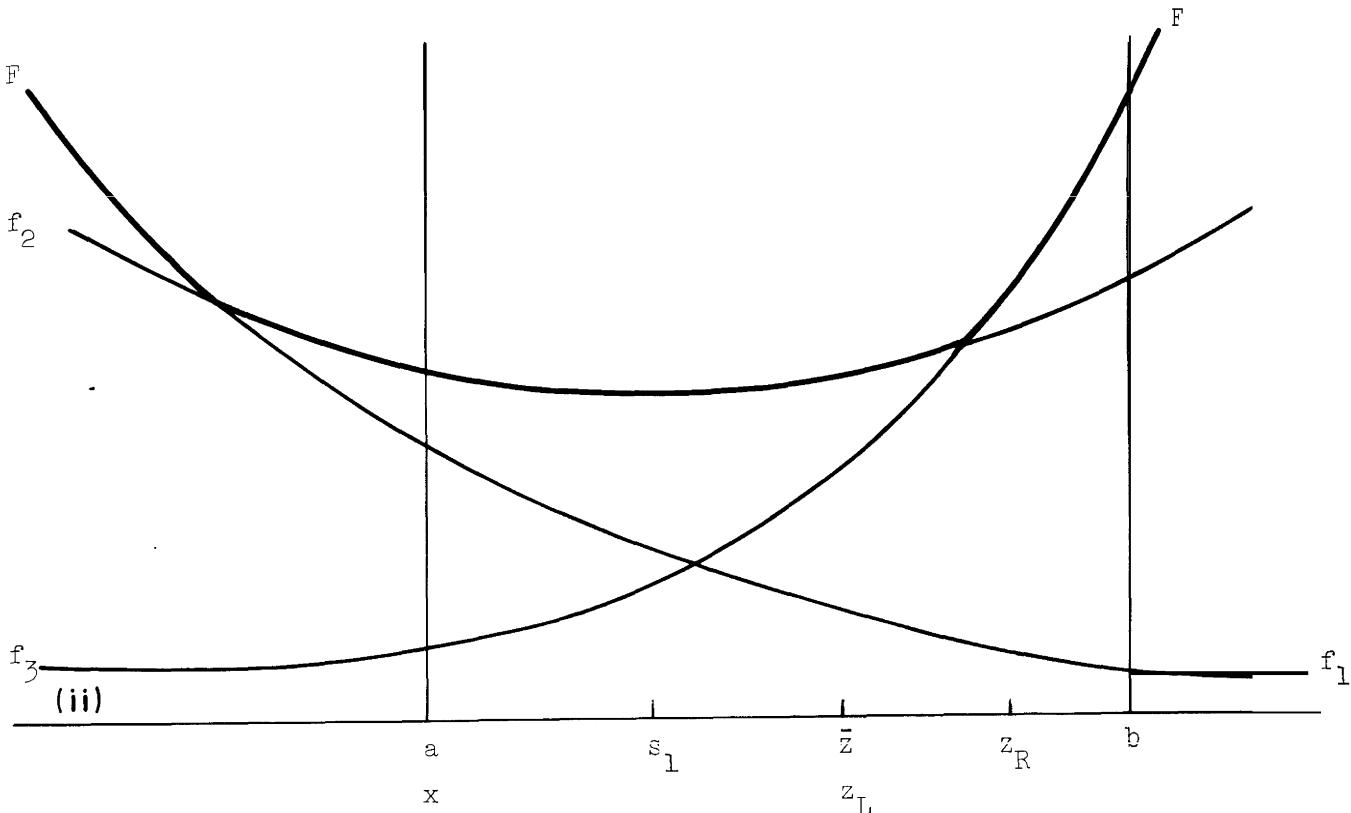
The step to  $s_1$ , the minimum predicted by the fit to  $f_2$ , is accepted.  $\hat{u}$  is set to  $s_1$ .
