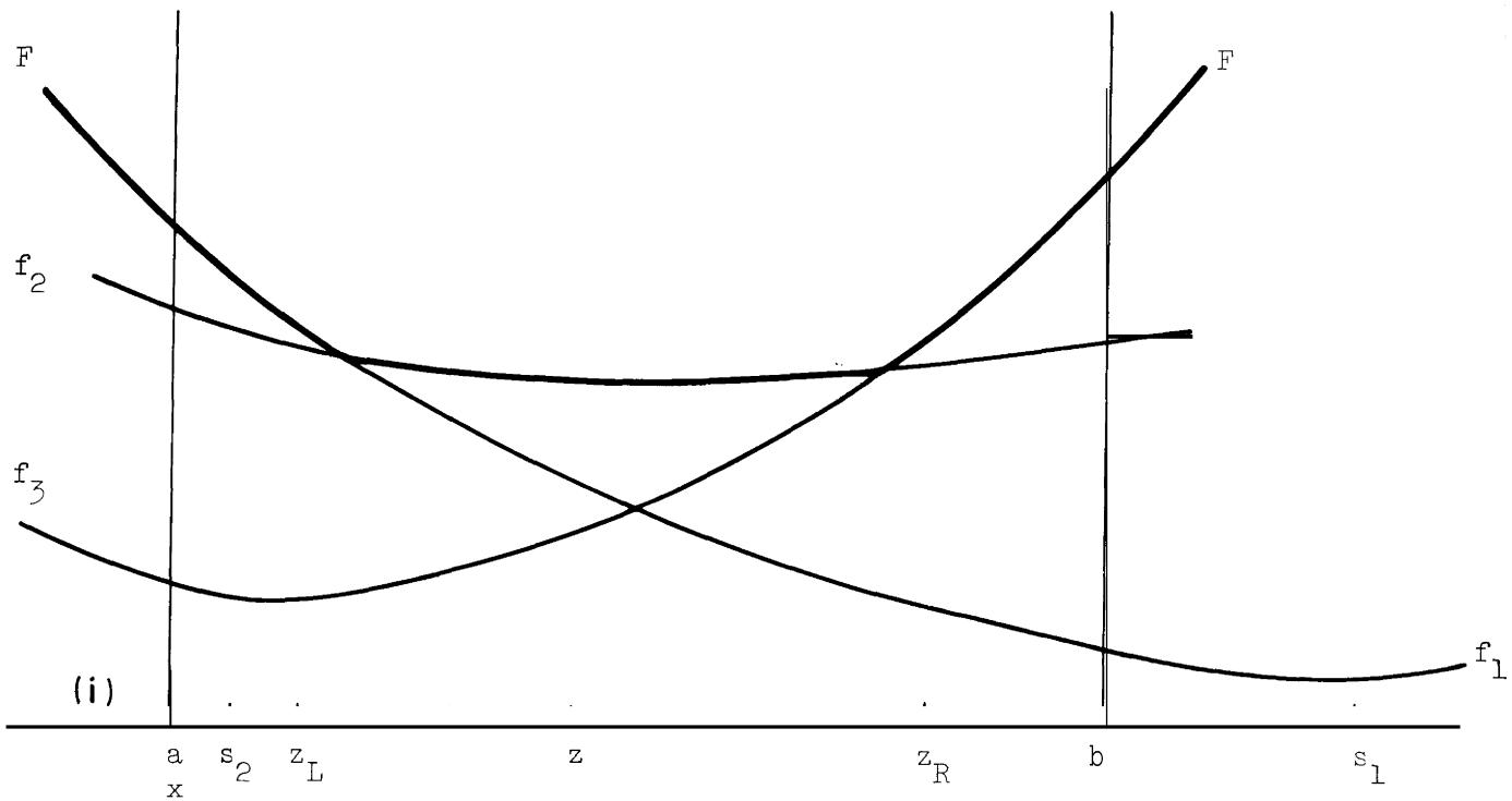
Determining  $\hat{u}$  for  $F = F_M$ . The step to  $s_1$ , the minimum predicted by the fit to  $f_1$ , and the step to  $s_2$ , the minimum predicted by the fit to  $f_3$ , are both rejected.  $\hat{u}$  is set to  $\bar{z}$
