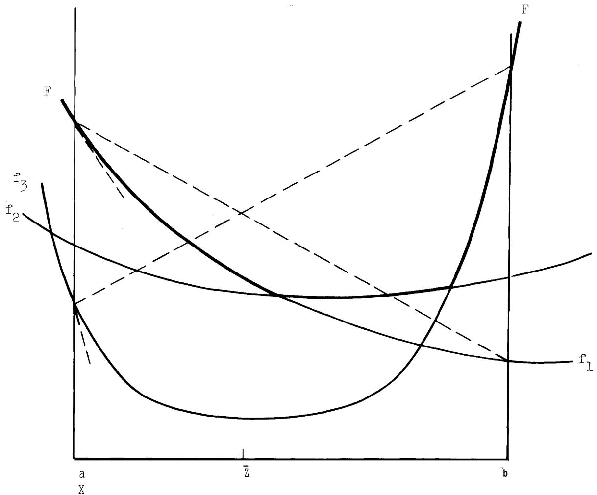
. Determining  $\bar{z}$  for  $F = F_M$ . The zero of  $f_1 - f_3$  is estimated. First the Newton step from  $x$  is tried, but since this lies outside  $[a,b]$  it is replaced by the secant step using  $a$  and  $b$ .
