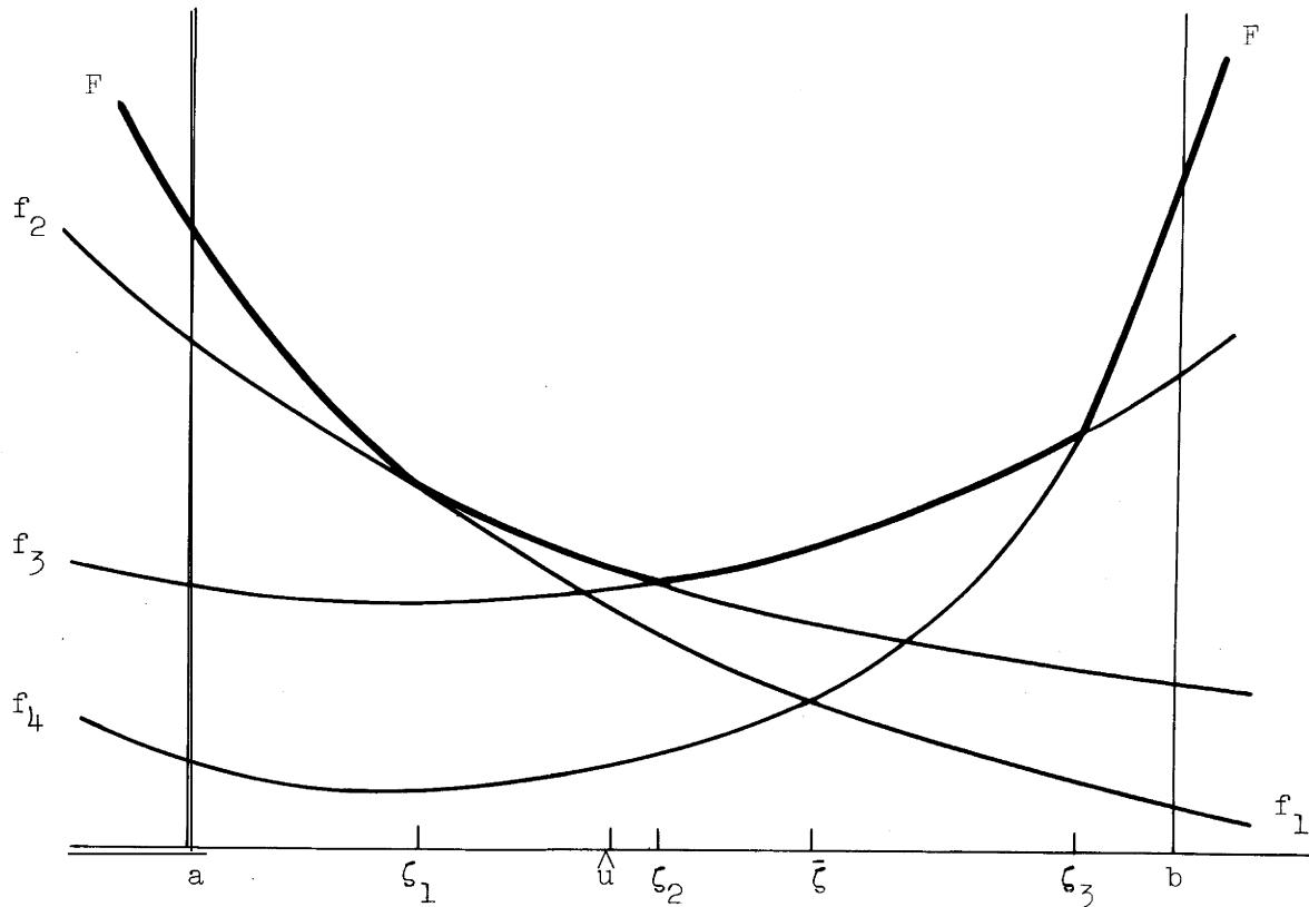
Determining  $\hat{u}$  for  $F = F_M$  in the higher overhead version. The zeros  $\zeta_1, \zeta_2, \zeta_3$  are successively estimated and the polynomial fits successively made to each function. Provided that the polynomial fit to  $f_2$  is decreasing to the right of the estimate of  $\zeta_2$  and that to  $f_3$  is decreasing to the left of it,  $\hat{u}$  is set to the estimate of  $\zeta_2$ . The low overhead version would have set  $\hat{u}$  to an estimate of  $\bar{\zeta}$ .
