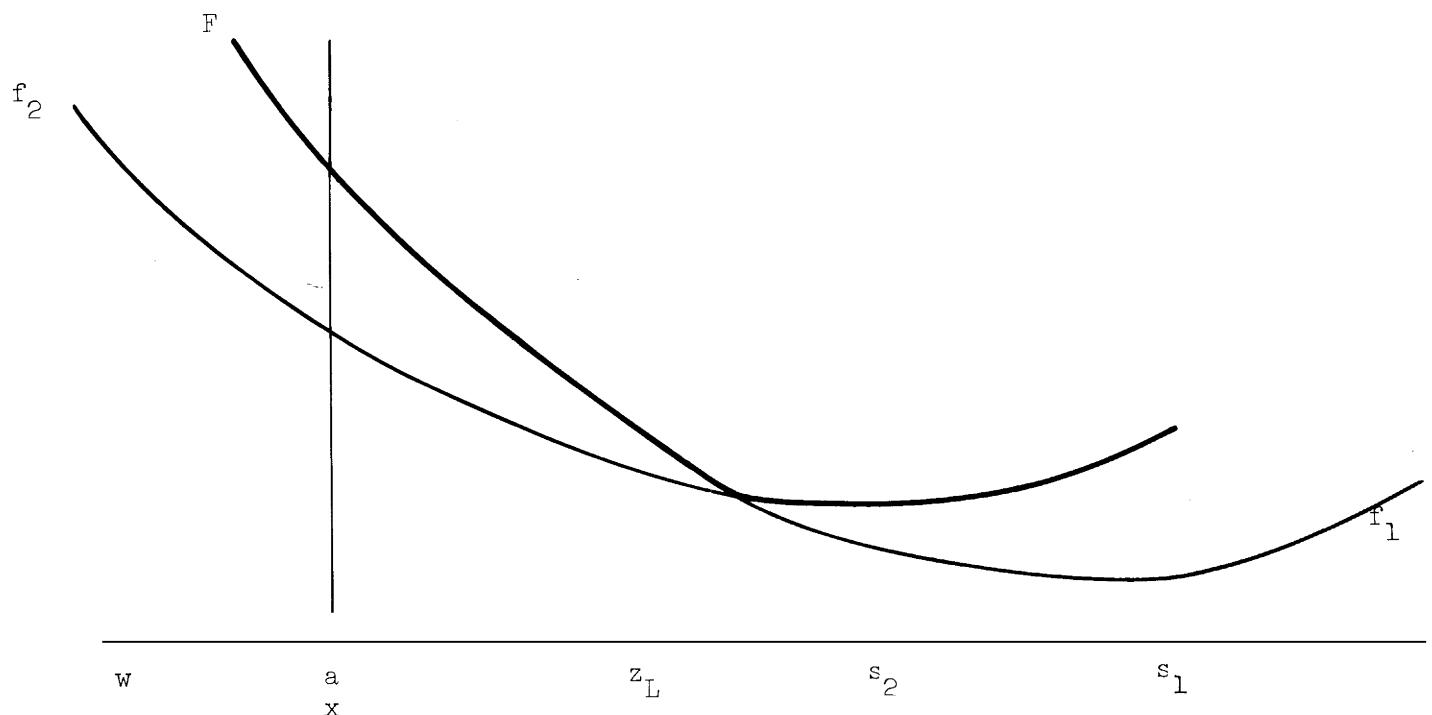
Determining  $\overset{A}{u}$  for  $F = F_M$  when the minimum is not bracketed. The step to  $s_1$ , the minimum predicted by the fit to  $f_1$ , is rejected, and so  $u$  is set to  $s_2$ , the minimum predicted by the fit to  $f_2$ .
