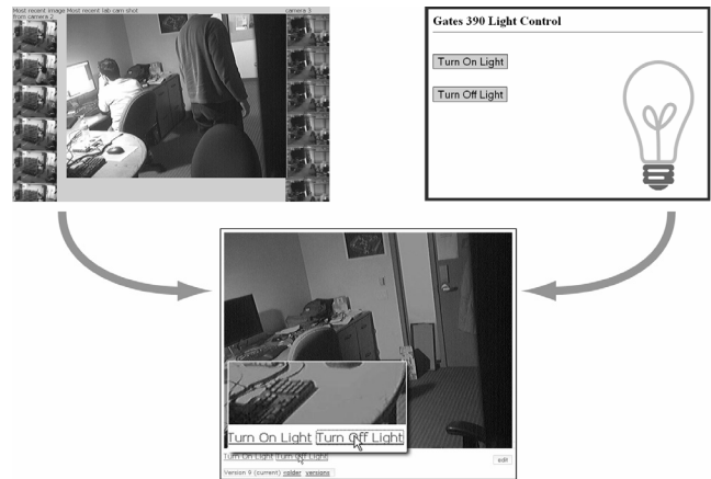
Figure 6. An example of a d.mix ubicomp mashup: web services provide video monitoring and lighting control.
