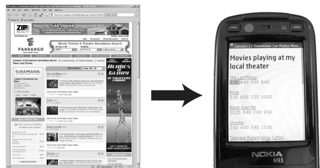
Figure 5. The rewriting technology in d.mix can be used to tailor content to mobile devices. Here, essential information is extracted from a movie listings page.
