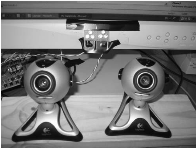
Figure 1: The low-cost prototype in development uses commercial-over-the-shelf cameras modified to work in the infrared spectrum. The glint source pictured above uses IR LEDs (invisible to the human eye).
