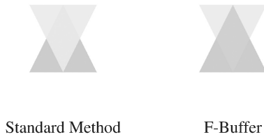
Figure 1: Here we use a simple example to show the difference between traditional multi-pass rendering using the framebuffer and using an F-Buffer when rendering transparent objects. We draw a cyan triangle behind a yellow triangle, each with an opacity of 0.5. We use a two pass shader that saves off the triangle colors in the first pass and restores the colors in the second pass. As is shown, the traditional method restores the values of the last fragments drawn for both triangles yielding incorrect results.
