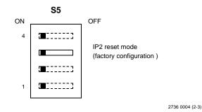
In IP2 mode, IP resets occur only in response to a direct software write or to a power-up reset; the IP reset control bit is not self-clearing.
