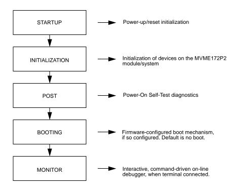
Figure 2-1. MVME172P2/Firmware System Startup
