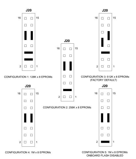
The next five tables show the address range for each EPROM socket in all four configurations. GPI3 (S4, switch segment 5) is a control bit in the MC2 General-Purpose Inputs register in the Petra ASIC that determines whether reset code is fetched from Flash memory or from EPROMs. (For
