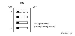
S5 varies in function according to the type of processor installed. For MVME162P2 boards with an MC68040 processor, setting segments 1 and 2 of switch S5 to **OFF** or leaving both segments set to **ON** (the factory configuration) inhibits snooping. Enabling snooping requires one of two possible **ON/OFF** combinations, according to the operation desired. MVME172P2 boards with an MC68060 processor have different snoop functionality.
