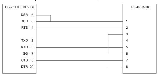
Figure 2-2. DB-25 DTE-to-RJ-45 Adapter
