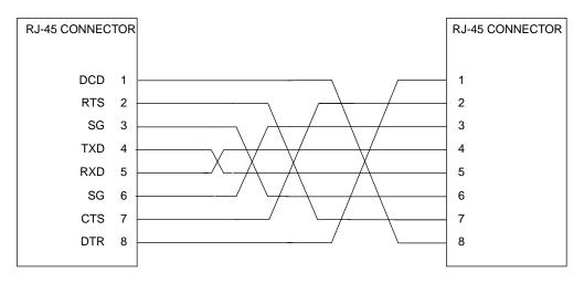
Figure 2-4. Typical RJ-45 Serial Cable
