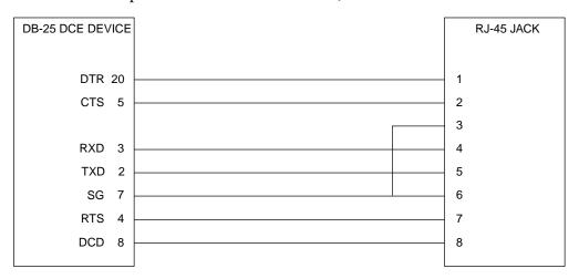
Figure 2-3. DB-25 DCE-to-RJ-45 Adapter
