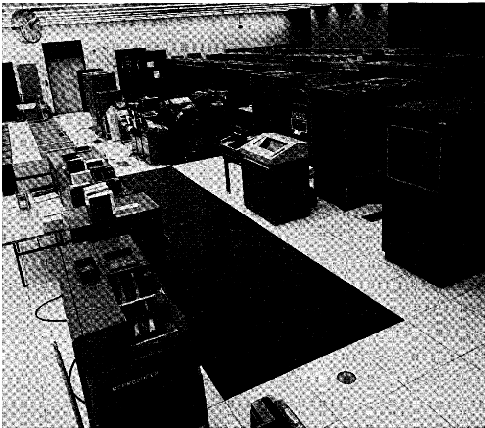
Some of the equipment at the Lawrence Livermore Laboratory computer complex; right center (with window) is part of the photodigital storage unit, left center are eight disc drives controlled by a PDP-10, behind the teletypewriters, and to the right are PDP-10 memories, PDP-8 concentrators, and assorted interfaces, including those for other computers in the network.
