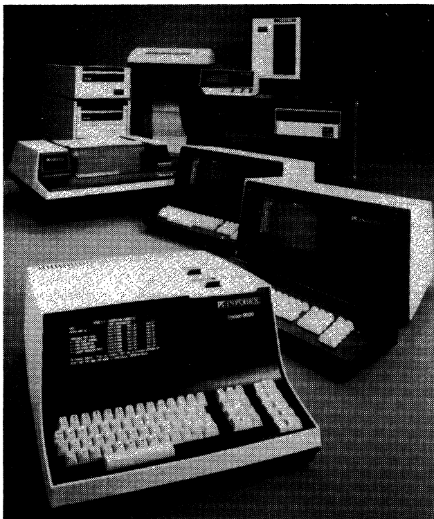
The System 9000 Distributed Information Processing System allows users to expand a local system or to grow into a local area network by adding a unit at a time. The system components that are shown here, starting from the foreground, are the system processor, Universal Workstation, matrix printer, disk storage systems, tape transport unit, and band printer.
