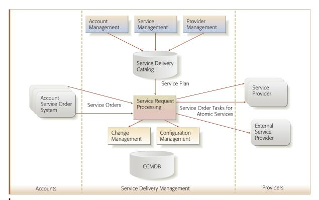
**Figure 1**Service delivery management architecture
