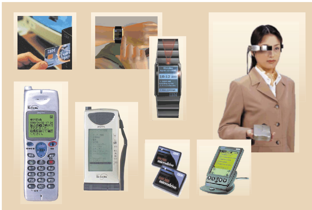
Figure 1 Sailing the “sea of devices.” Shown here (clockwise from top left) are smartcards as an example of a pervasive authentication token, IBM's Watchpad (two images), an IBM wearable computer prototype, the Palm Pilot™ as an example of a connected personal digital assistant, two IBM microdrives, and two i-mode smart phones.
