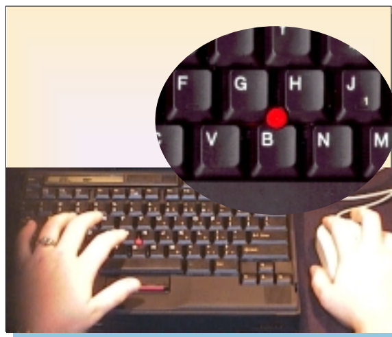
Figure 4 In-keyboard isometric joystick (top), operated by the nondominant hand (left for this user) for scrolling while the dominant hand moves a mouse for pointing (bottom)
