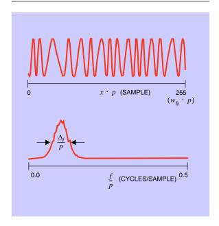
and  $\Delta_f$  in spatial frequency) determine the information content of the encoded fringe. Hogel-vector encoding reduces the number of symbols by sampling hogel spectra in large frequency steps. The amount of bandwidth compression in an encoded fringe is measured by the compression ratio, CR:
