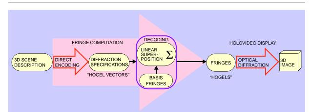
Figure 1 Hogel-vector bandwidth compression: direct encoding and decoding using superposition of precomputed basis fringes
