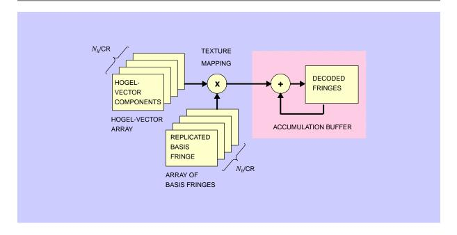
decoded in the RE2, as shown in Figure 10. The texture-mapping function rapidly multiplied a component from each hogel vector by a replicated array of a single basis fringe. This operation is repeated  $N_h$  / CR times, once for each hogel-vector component, accumulating the result in the accumulation buffer. Transfer times were negligible because all computations occurred inside the graphics subsystem that included
