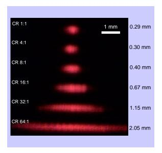
with  $\Delta_f$ . For CR = 8:1 or less, the point is still sharp. For CR = 16:1, the effective width increases such that it is easily seen by a human viewer. Hogel width was  $N_h = 512$  samples or  $w_h = 0.3$  mm.
