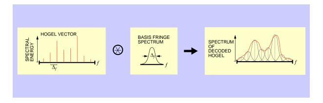
By encoding the 3D scene description as diffraction specifications—an array of hogel-vectors—this technique reduces required bandwidth. Speed results from the simplicity, efficiency, and directness of basisfringe summation in the decoding step.
