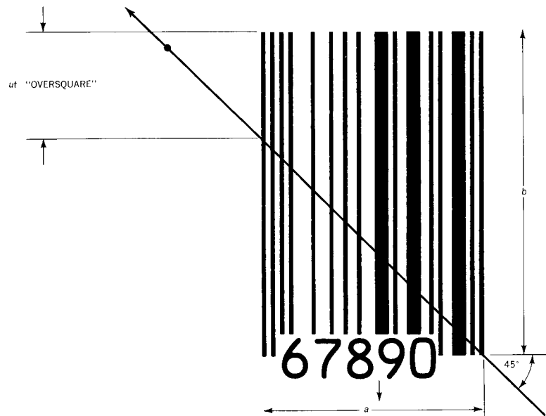
Figure 10 Dimensional parameters for omnidirectional scanning
