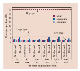
Resistance for interlevel vias through areas with and without bonded interface for chains with various via numbers, showing that the quality of the bonded interface is good and does not degrade the electrical performance of the device-connecting vias for all via-chain lengths tested (resistance within the expected value <4  $\Omega$  per link). Reprinted from [32] with permission; ©2005 IEEE.
