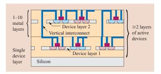
Schematic diagram of three-dimensional integrated circuit (3D IC) showing two stacked device layers with their corresponding metallization levels and inter-device-layer connections (vertical interconnects). Reprinted from [16] with permission; ©2002 IEEE.
