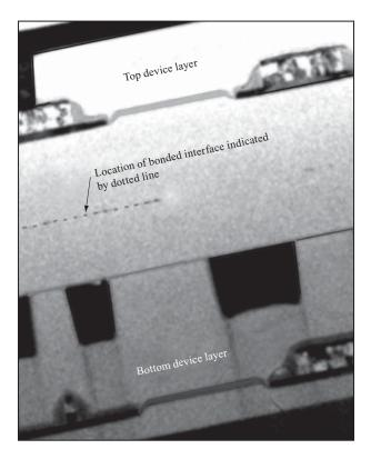
Cross-sectional TEM image of two metallized, stacked, and oxide-fusion-bonded SOI CMOS device layers.
