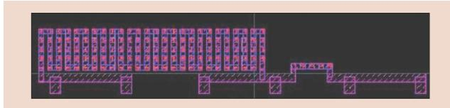
3D via-chain diagram for resistance characterization testing 128 interlevel vias (left) and four-via structure (right), providing reliability and yield learning about high-aspect-ratio 3D interlayer vias. Reprinted from [34] with permission; ©2005 IEEE.
