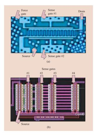
(a) Top-down optical image of a fabricated 28-finger n-FET for self-heating measurement in 3D ICs; (b) schematic diagram of five FETs on each wafer in a 3D chip for measuring temperature rise due to spread-heating. Reprinted from [39] with permission.
