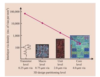
Schematic diagrams of applications for 3D integration based on 3D partitioning level and the required interlayer via density. (Personal communication with R. Puri, IBM Research Division, 2005.)
