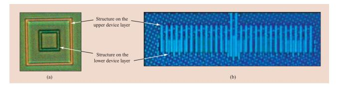
(a) 3D box-in-box bonding alignment structure showing nearly perfect alignment ( $<0.2 \mu m$ ); (b) top-down optical image of fabricated Vernier grids. The minimum achievable resolution with a Vernier structure is 0.18  $\mu m$ . Reprinted from [32] with permission; ©2005 IEEE.
