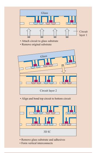
Schematic diagrams of IBM assembly process, which uses layer transfer methodology to fabricate 3D ICs. Reprinted from [16] with permission; ©2002 IEEE.
