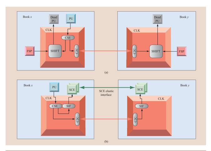
Run-control functions executed by a PU: (a) PU sparing operation. (b) L2 ring unfencing sequence. (C2C: clock to clock; CLK: clock chip; CSE: clock support element; FSP: flexible service processor; PU: processing unit; SCE: service control element; SIF: serial interface.)
