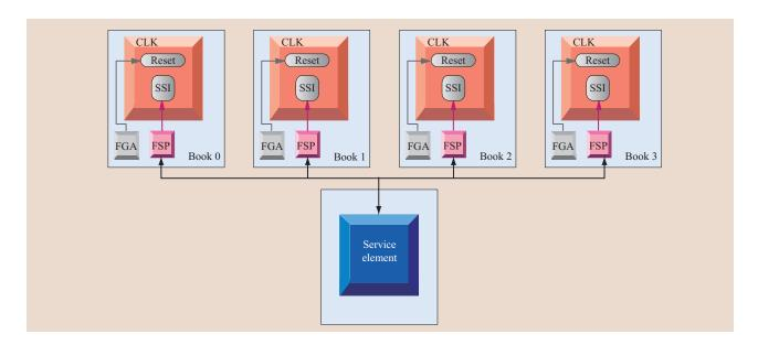
System structure of a four-book system. Only active FSPs are shown. (CLK: clock chip; FGA: field gate array chip, which provides reset signals to the clock chip; FSP: flexible service processor; SSI: system support interface.)
