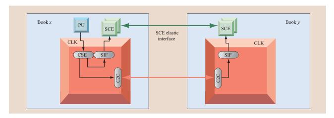
L2 ring unfencing sequence. (C2C: clock to clock; CLK: clock chip; CSE: clock support element; PU: processing unit; SCE: system control element; SIF: serial interface.)
