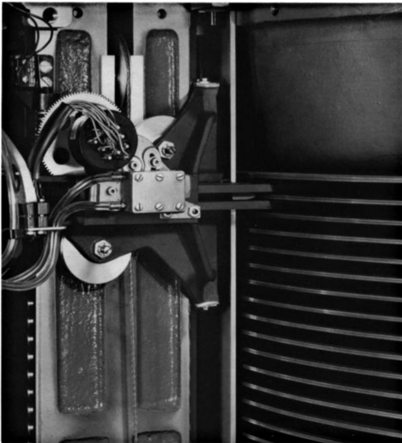
Figure 1 Access mechanism of the IBM Type 350 magnetic-disk, random-access memory.
