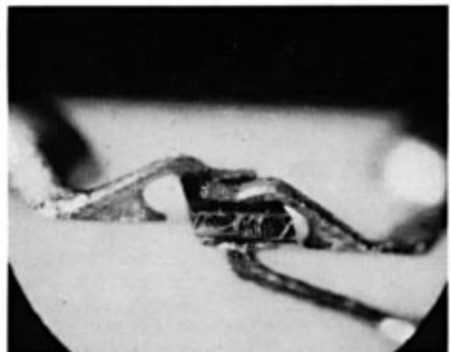
Figure 17 Mounting technique for power device.
