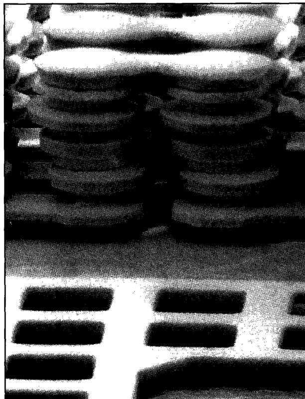
SEM photograph showing a via stack with 11 levels of metallurgy. (Polyimide has been ashed away as in Figure 3.)
