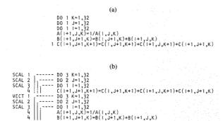
Vectorization of loop with recurrences: (a) original source program; (b) vectorized program.
