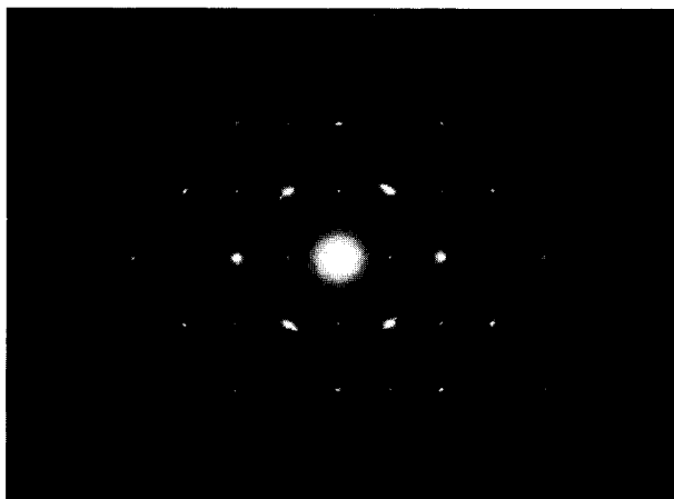
Figure 9 Electron diffraction pattern from the basal plane of PHBA. The molecular weight of this specimen was greater than 50 000, but similar diffraction patterns were obtained from tetramer and higher in molecular weight.
