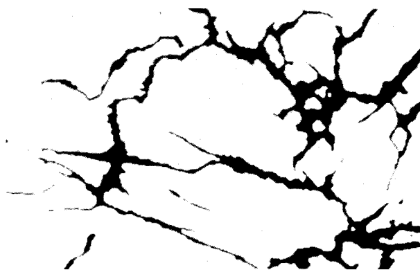
Figure 3 Binary image from Fig. 2(a) with the fissure network.
