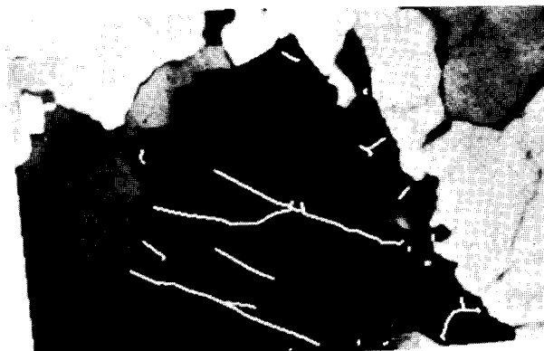
Figure 11 Fissures contained in grain no. 3, from which a fissuration density is calculated. Only one intragranular fissure of length 0.33 mm is visible in the center of the lower part of the grain; all other fissures are portions of transgranular ones.
