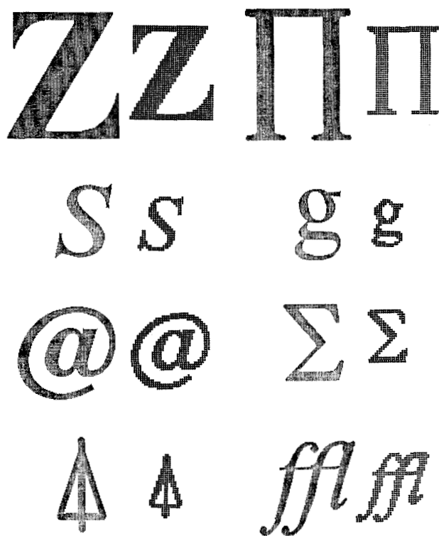
Figure 8 Photocomposer (high-resolution) characters scaled to 240 pixels/inch. Characters that are ordinarily thought of as symmetrical, e.g., "pi," are often not symmetrical at photocomposer resolutions (here 800 pixels/inch). Thus the scaled version is not pixel-for-pixel symmetrical.
