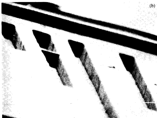
Figure 16 Overlay of two exposures at 50% dose each. (a) Positional inaccuracies not compensated. (b) Positional inaccuracies automatically compensated through beam tilting. At the bottom of the picture are 1-μm calibration marks.
