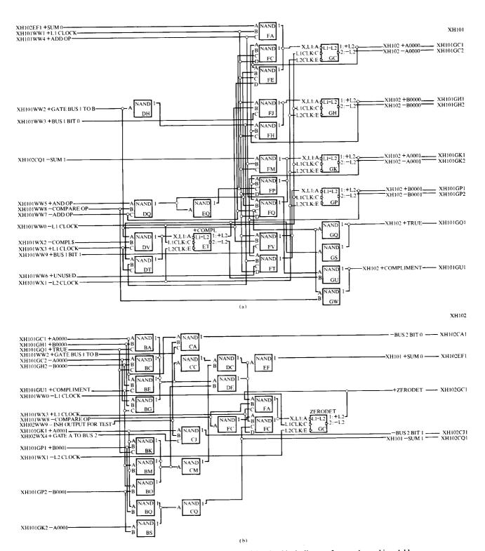
Figure 5 (a) Low-level logic diagram for sample machine: Registers; (b) low-level logic diagram for sample machine: Adder.
