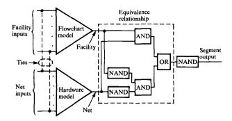
Figure 6 Basic segment structure.
