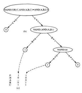
Figure 7 Examples of differential Boolean analyzer (DBA): (a) segment model; (b) tree; (c) counterexamples.
