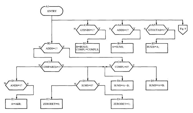
Figure 2 Hardware flowchart for sample machine.
