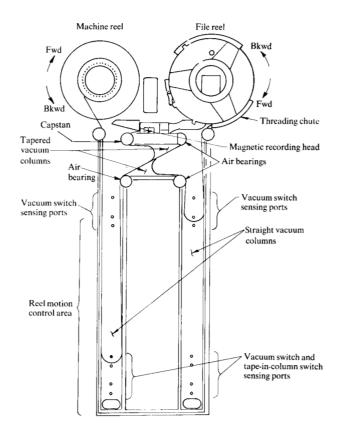
Figure 5 Tape path for the IBM 2420 Model 7.
