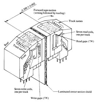
Figure 3 The two-gap, seven-track head used in the IBM 729. The combination of separate read and write heads permitted read checking immediately after writing.
