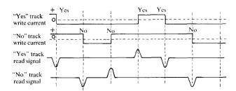
Figure 2 The NRZI code, in which the "yes" track and "no" track guarantee a translation per bit to permit self-clocking.
