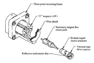
Figure 4 Exploded view of the high-torque, low-inertia motor.
