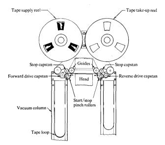
Figure 1 Tape drive utilizing pinch roller.
