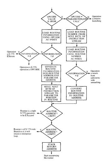
Figure 3 Operation decoding by the interpreter.
