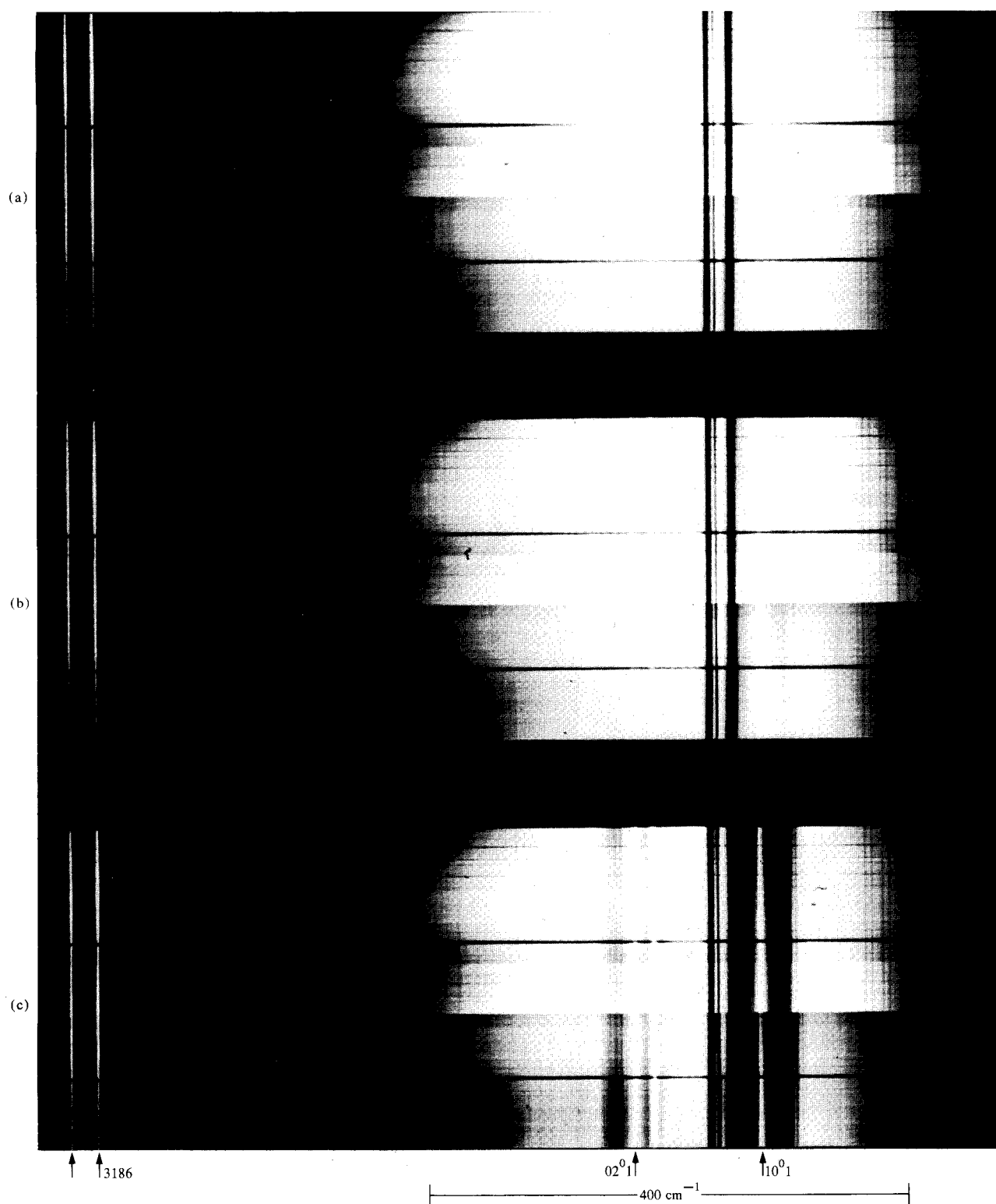
Figure 4 Upconverted DPS K-K spectrum (first order) with sample cell (a) evacuated, (b) containing a small unmeasured amount of \text{CO}_2 , and (c) containing \approx 67 kPa (500 torr) \text{CO}_2 . In all three cases two exposures are shown.
