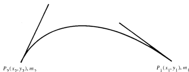
Figure 1 A cubic can be defined by the points P_1(x_1, y_1) and P_2(x_2, y_2) where the associated slopes are m_1 and m_2 , respectively.
